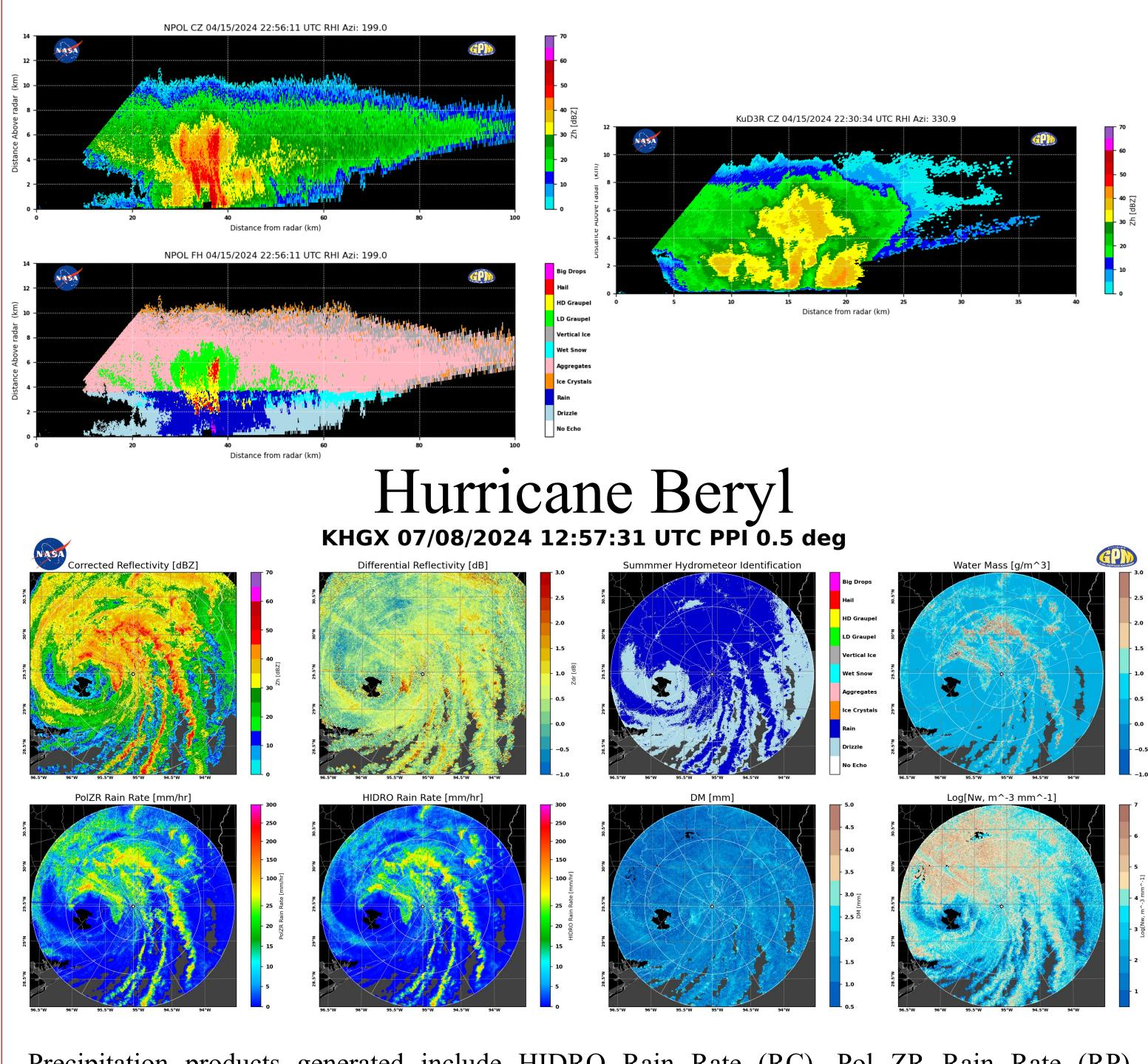
Precipitation products generated include HIDRO Rain Rate (RC), Pol ZR Rain Rate (RP), Hydrometeor Identification (FH), Ice and Liquid mass (MI, MW), mass weighted mean diameter (Dm), and normalized intercept parameter (Nw).
